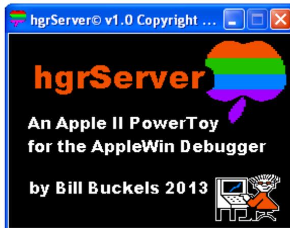
hgrServer is a very simple program. It is not an application or even a utility. All it does is runs in the background and renames default filename and numbers them sequentially while you merrily BSave HGR Screens in the AppleWin debugger using the debugger's default naming.
